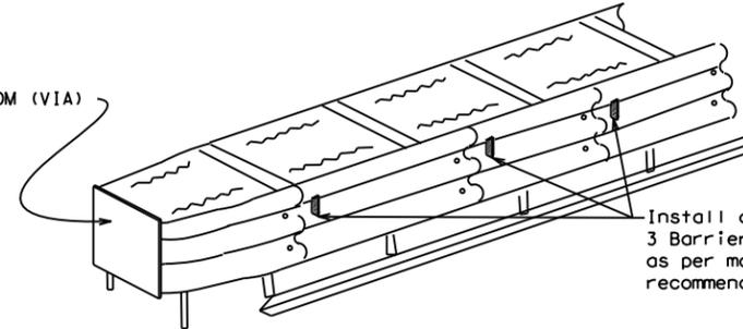
Install a minimum of 3 Barrier Reflectors as per manufacturer's recommendations.
