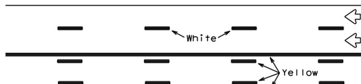
REFLECTORIZED PAVEMENT MARKINGS
