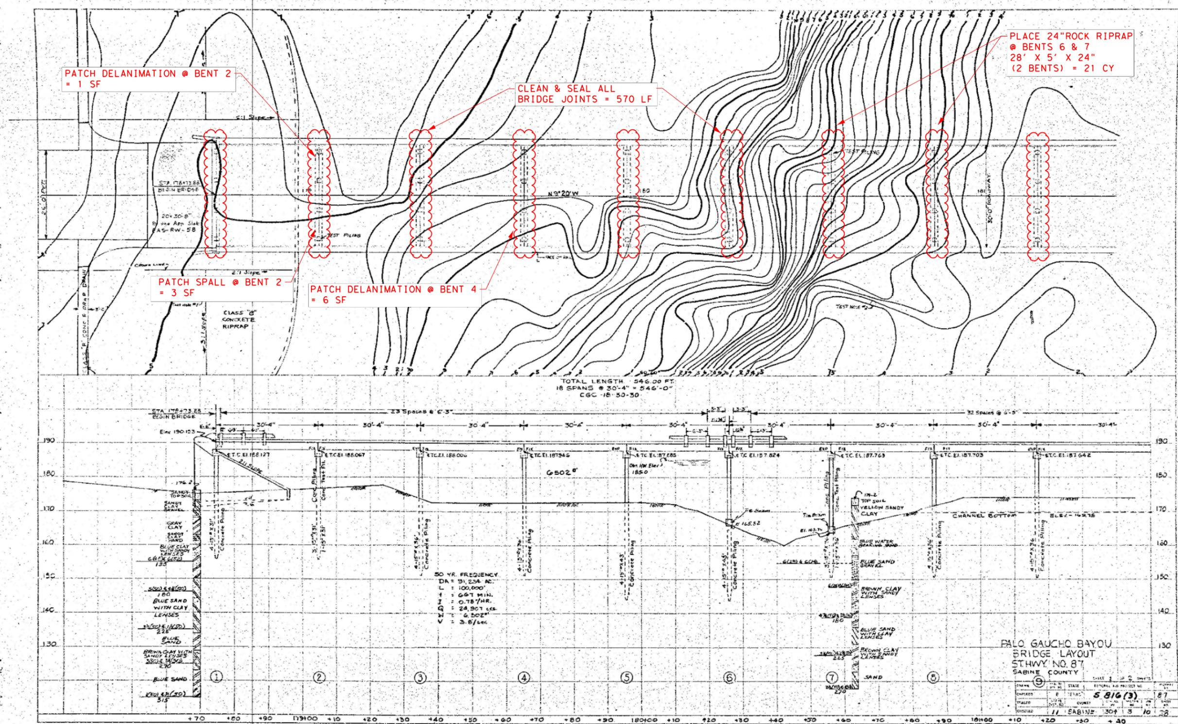
NOTE: CLEANING AND SEALING OF EXISTING JOINTS SHALL BE PERFORMED DURING THE COOLER MONTHS TO AVOID EXCESS EXPANSION AS DIRECTED BY THE ENGINEER
