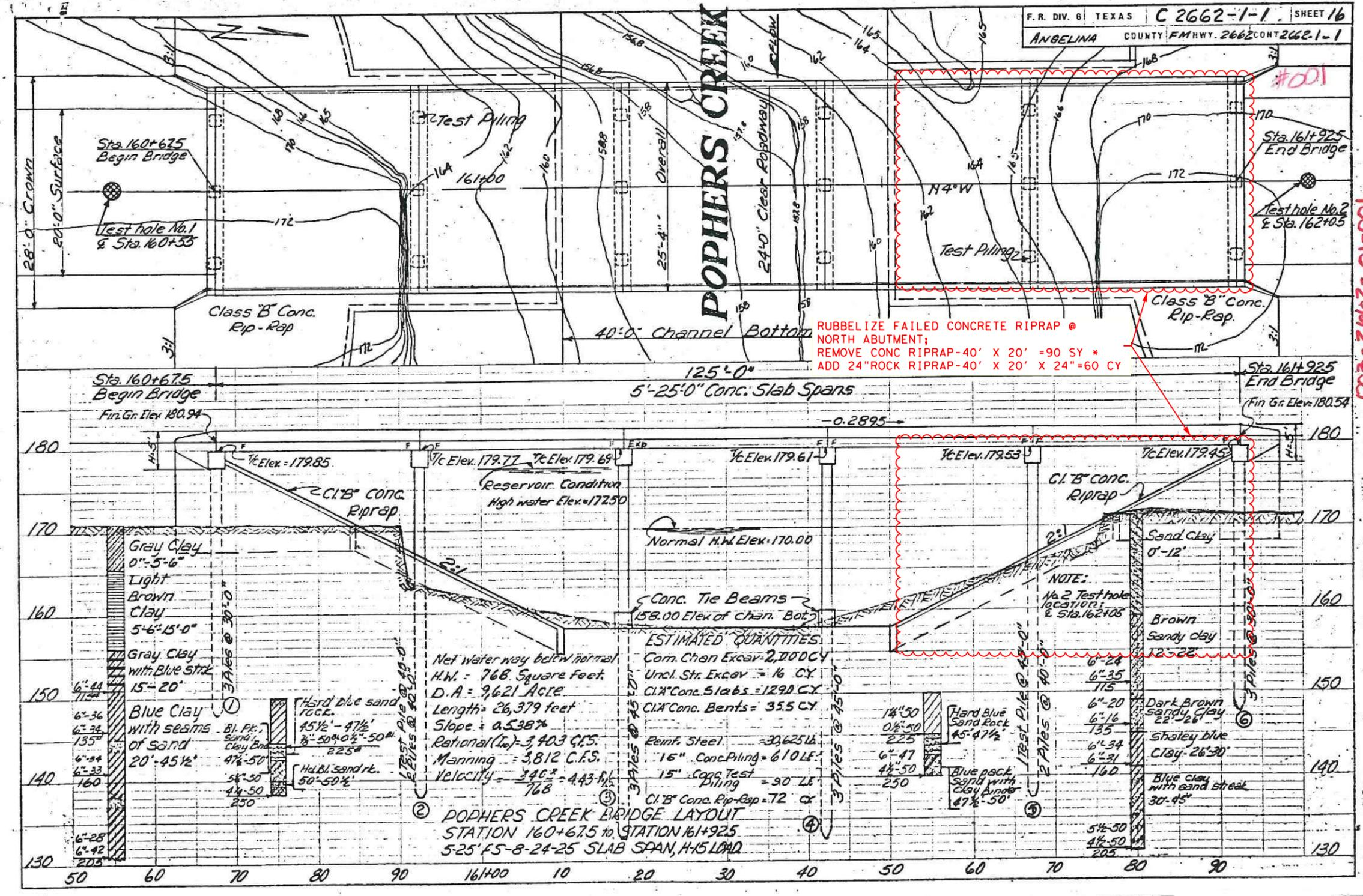
RUBBERIZE FAILED CONCRETE RIPRAP @ NORTH ABUTMENT; REMOVE CONC RIPRAP-40' X 20' = 90 SY \* ADD 24" ROCK RIPRAP-40' X 20' X 24" = 60 CY
