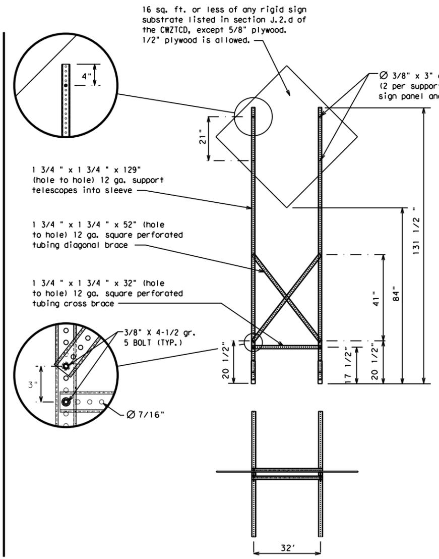
**SKID MOUNTED PERFORATED SQUARE STEEL TUBING SIGN SUPPORTS**
