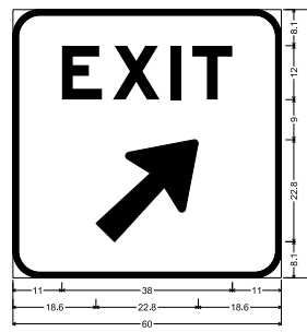
6.0" Radius, 1.3" Border, White on, Green: "EXIT", E Mod; Arrow 16 - 29.0" 45";
