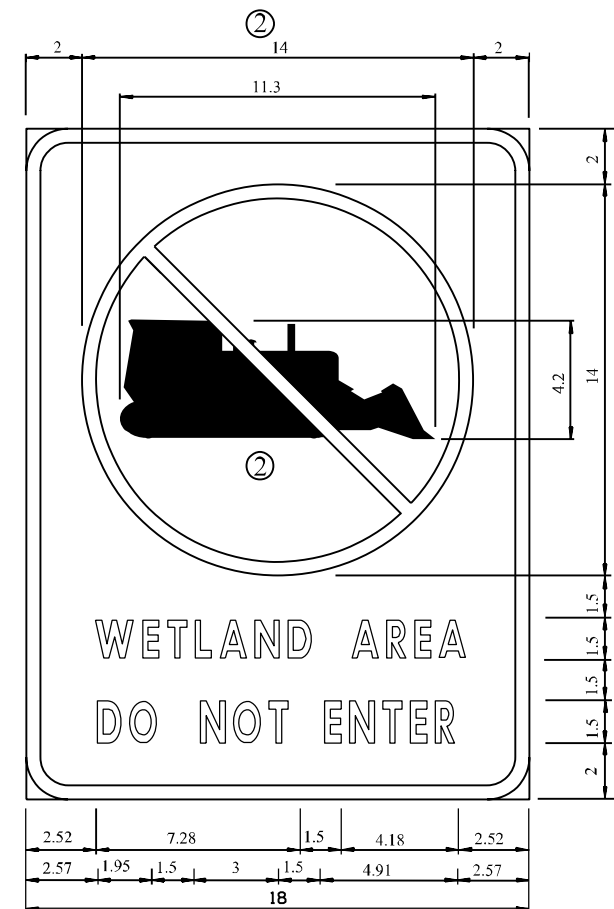
1.50" Radius, 0.50" Border, Black on White; [WETLAND AREA] C; [DO NOT ENTER] C; CIRCLE, DIAG LINE, RED
