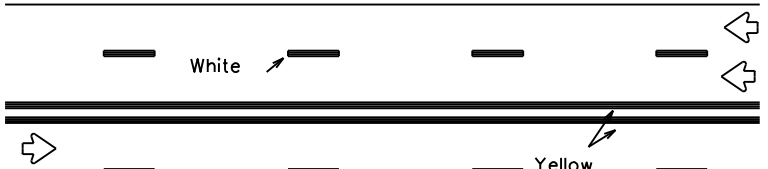
REFLECTORIZED PAVEMENT MARKINGS
