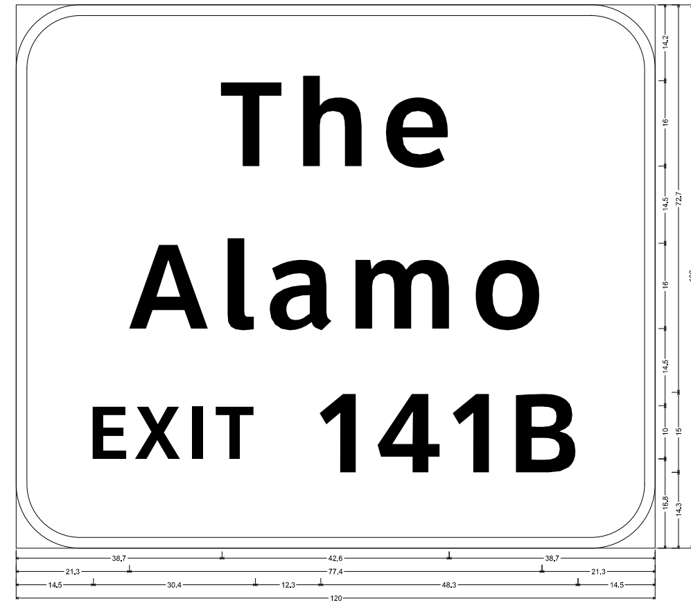
120x102: 12.0" Radius, 2.0" Border, White on, Brown: "The", ClearviewHwy-5-W-R; "Alamo", ClearviewHwy-5-W-R; "EXIT 141B", ClearviewHwy-5-W-R;
