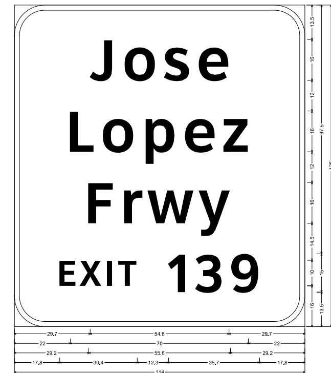
114x128: 12.0" Radius, 2.0" Border, White on, Brown: "Jose", ClearViewHwy-S-W-R; "Lopez", ClearViewHwy-S-W-R; "Frwy", ClearViewHwy-S-W-R; "EXIT 139", ClearViewHwy-S-W-R;
