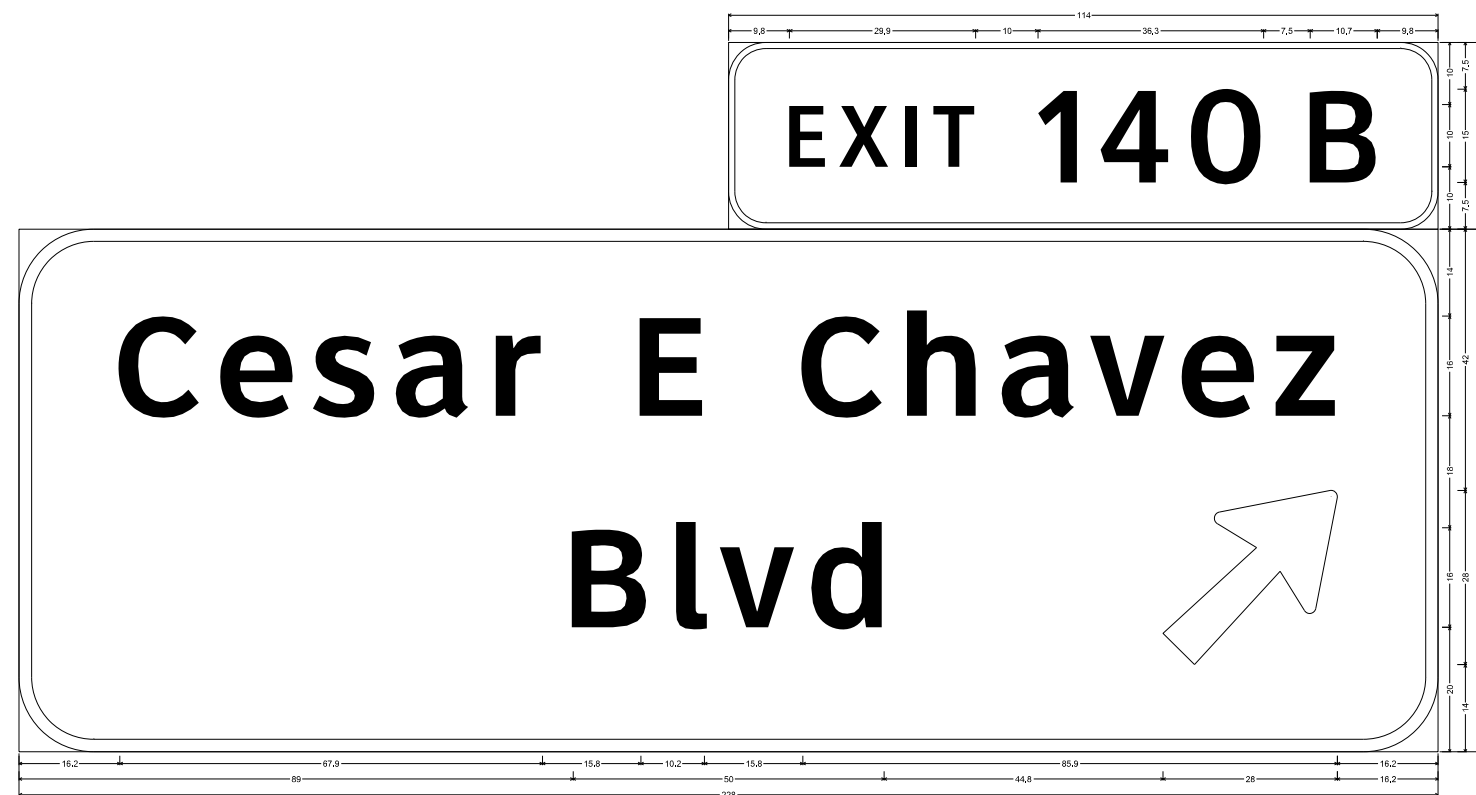
228x114: E14R_114x30: 6.0" Radius, 1.0" Border, White on, Green: "EXIT 140", ClearViewHwy-W-R; "B", ClearViewHwy-W-R specified length; 12.0" Radius, 2.0" Border, White on, Green: "Cesar E Chavez", ClearViewHwy-S-W-R; "Blvd", ClearViewHwy-S-W-R; Arrow A-3 = 35.6" AS
