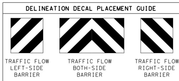
NOTE: APPLY A HIGH REFLECTIVE DECAL TO THE NOSE PLATE. DELINEATION DECAL ORIENTATION IS SHOWN ON THE CONSTRUCTION PLAN SET AND SHALL BE IN ACCORDANCE WITH THE TEXAS MUTCD FOR (TRAFFIC CONTROL DEVICES). DECALS ARE AVAILABLE FOR TRAFFIC FLOW ON THE LEFT-SIDE, BOTH -SIDES AND RIGHT-SIDE.
