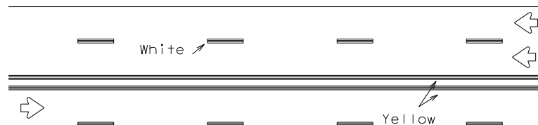
REFLECTORIZED PAVEMENT MARKINGS
