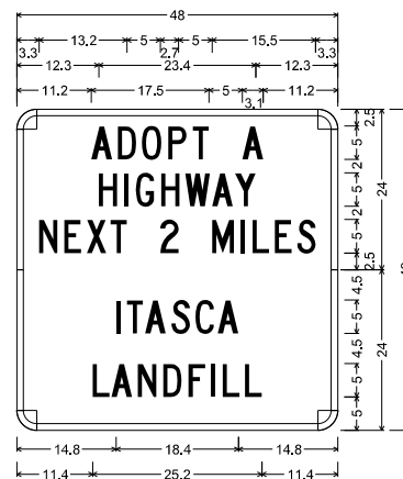
D14-4T-2_48x48: 3.0" Radius, 1.0" Border, White on, Blue; "ADOPT A", C; "HIGHWAY", C; "NEXT 2 MILES", C; 3.0" Radius, 1.0" Border, White on, Blue; "ITASCA", C; "LANDFILL", C;
