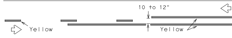
REFLECTORIZED PAVEMENT MARKINGS - PATTERN A
