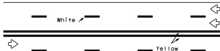
REFLECTORIZED PAVEMENT MARKINGS
