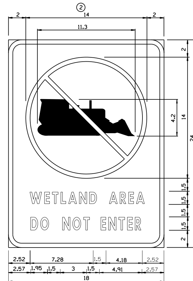
1.50" Radius, 0.50" Border, Black on White; [WETLAND AREA] C; [DO NOT ENTER] C; CIRCLE, DIAG LINE, RED
