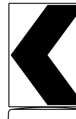
18" x 24" Sign (Maximum Sign Dimension) Chevron CWI-8, Opposing Traffic Lane Divider, Driveway sign D70a, Keep Right R4 series or other signs as approved by Engineer
