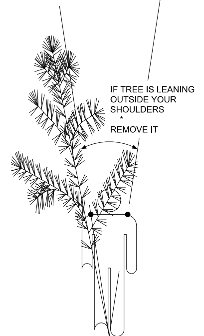
LEANING TREE REMOVAL
