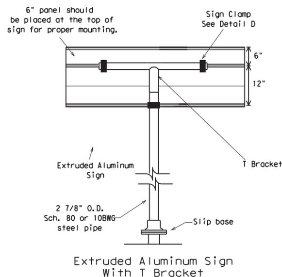
Use Extruded Alum. Windbeam as stiffeners See SMD (2-1) for additional details
