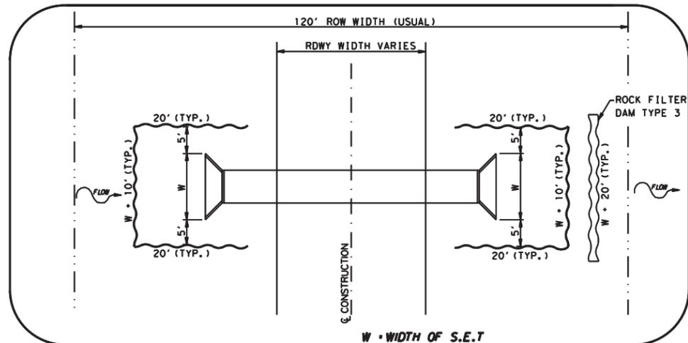
**2 SILT FENCE DETAIL FOR CROSSING STRUCTURES ON ROADWAY**
