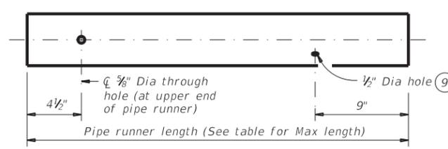
NOTE: The separate pipe runner shown is required when Cross Pipe Connection Option A1 is used.
