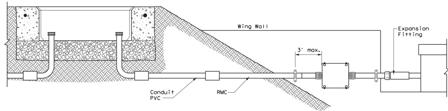
TYPICAL CONDUIT ENTRY TO BRIDGE STRUCTURE DETAIL
