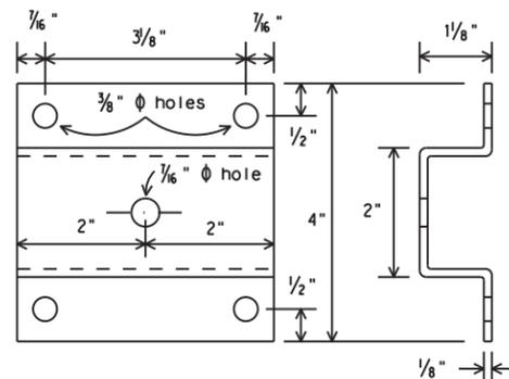
Wing channel, 4" width x 1/8" depth x 1/8" thickness, shall be aluminum (ASTM B221 6061-T6 or B308 6061-T6), galvanized steel (ASTM A36) or stainless steel (ASTM A167 type 304, No. 2B finish).
