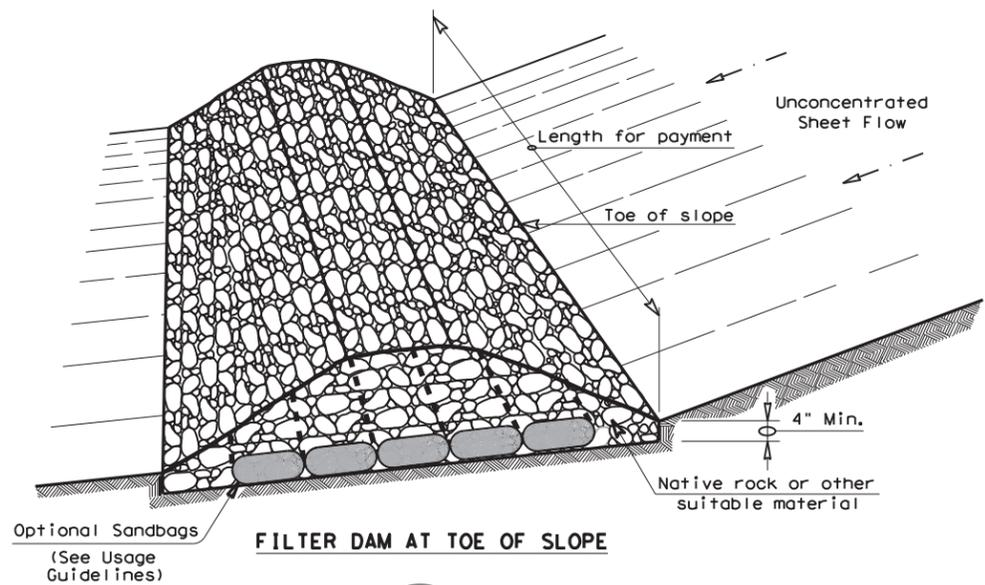
**FILTER DAM AT TOE OF SLOPE**
