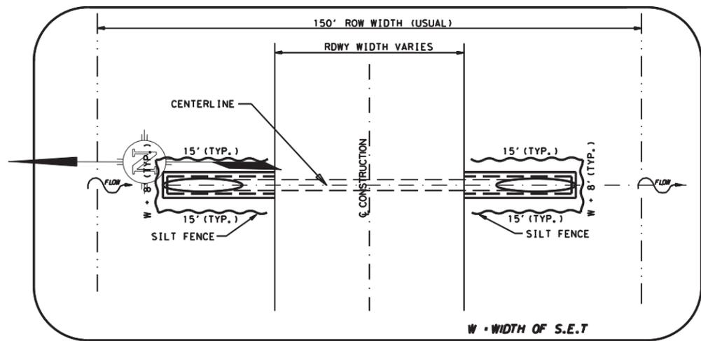
**1 SILT FENCE DETAIL FOR PIPE ON ROADWAY**
