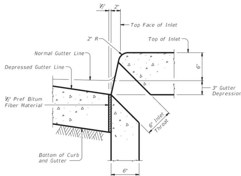
**SECTION AT GUTTER AND INLET**
