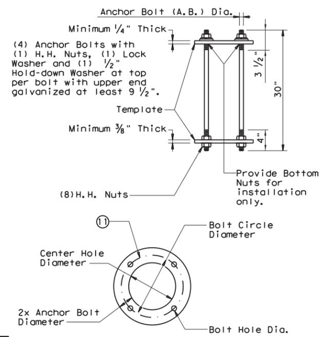
**TRANSFORMER BASE ANCHOR BOLT ASSEMBLY**
