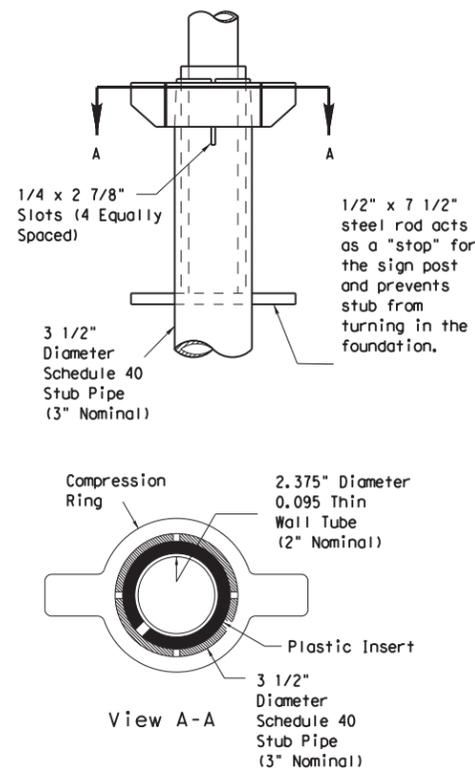
Plastic insert must be used when using the TWT with either the Universal Anchor System or the Bolt Down Universal Anchor System. The insert should be approx. 10" long and cover the tubing from just above the top of the stub pipe to the bottom of the sign post when using the Universal Anchor System. The insert should be cut to approx. 4 1/2" when used with the Bolt Down Universal Anchor System.
