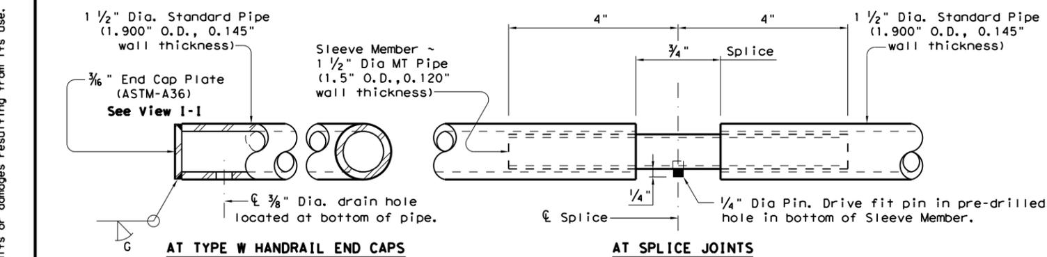
**HANDRAIL FABRICATION DETAILS**
