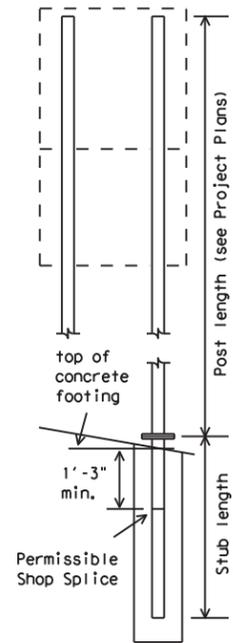
The weight of one S4x7.7 post is equal to 112.2 lbs. plus 7.7 lbs./ft x (post length in feet minus 10 ft). The weight of 112.2 lbs. includes 10 feet of post length, post foundation stub, related connection plates, friction fuse plate, and all high strength bolts, nuts and washers.
