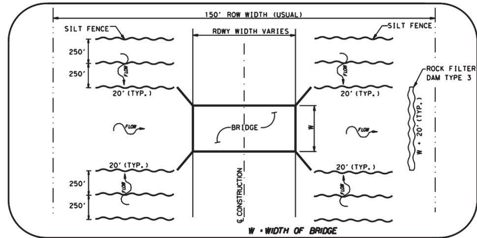
**3 SILT FENCE DETAIL BRIDGE ON ROADWAY**
