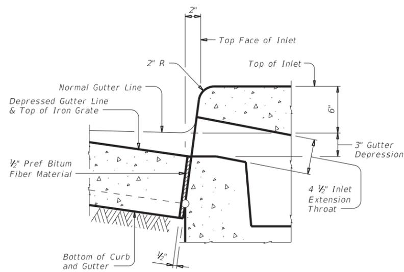
**SECTION AT GUTTER AND INLET**
