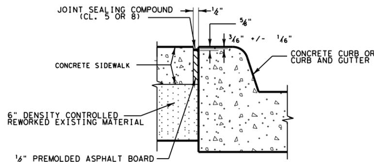
**3 1/2" ISOLATION JOINT (N.T.S.) (SIDEWALK ADJACENT TO CURB)**
