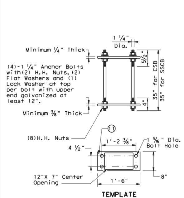
**CONCRETE TRAFFIC BARRIER BASE ANCHOR BOLT ASSEMBLY**
