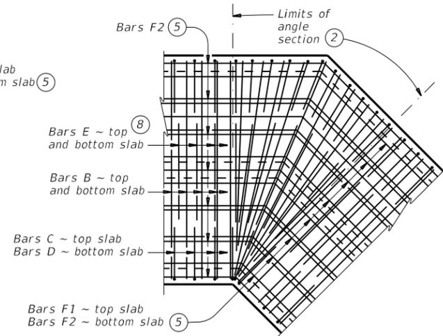
**PLAN OF ANGLE SECTION ~ OVER 30° TO 45°**
