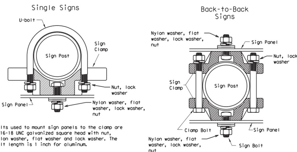
Bolts used to mount sign panels to the clamp are 5/16-18 UNC galvanized square head with nut, nylon washer, flat washer and lock washer. The bolt length is 1 inch for aluminum.
