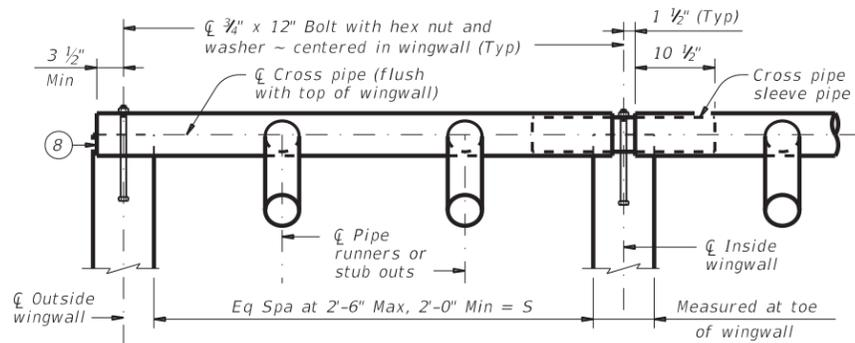
NOTE: At Contractor's option, make the cross pipe continuous across the inside wingwalls. If option is selected, omit the sleeve pipe and make a 1 5/16 inch diameter through hole in the cross pipe to accept the anchor bolt at the centerline of each inside wingwall.
