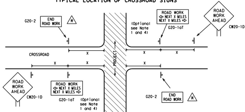
⚠ May be mounted on back of "ROAD WORK AHEAD" (CW20-1D) sign with approval of Engineer. (See note 2 below)
