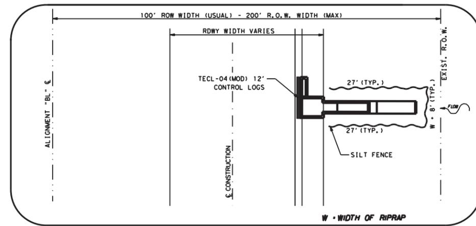
**4 SILT FENCE DETAIL FOR INLET W/RIPRAP ROADWAY**
