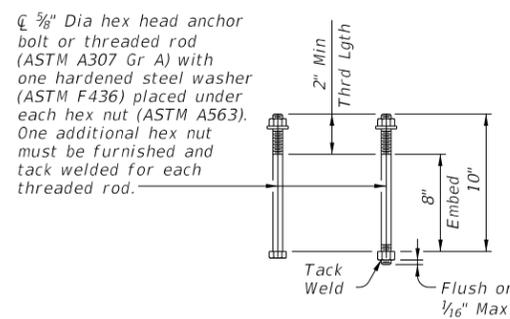
**CAST-IN-PLACE & FORMED HOLE ANCHOR BOLT OPTIONS**
