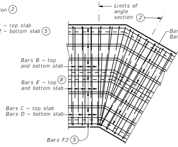
**PLAN OF ANGLE SECTION ~ OVER 15° TO 30°**
