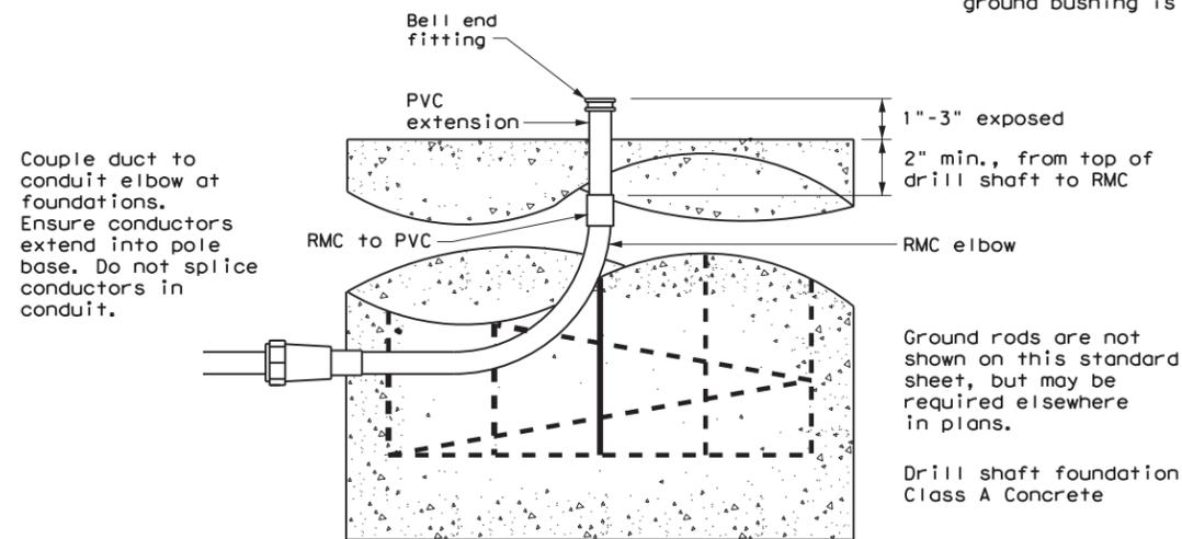
**DUCT CABLE / HDPE AT FOUNDATION**
