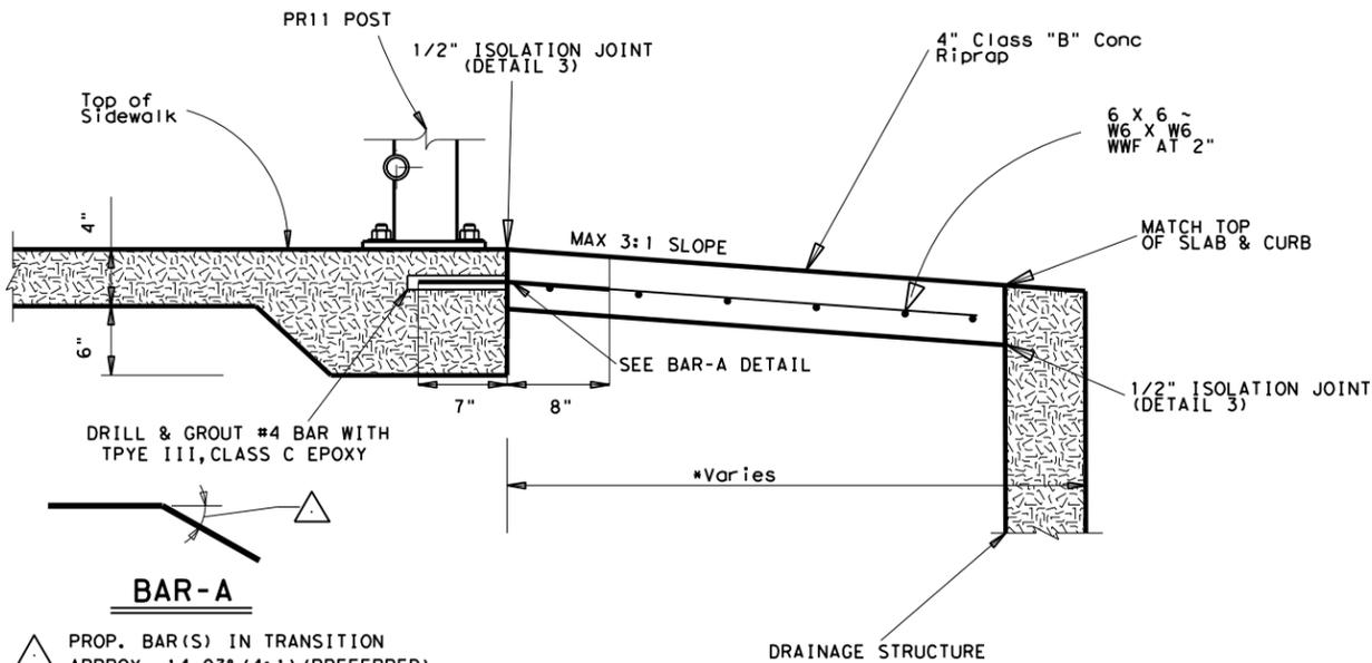
**RIPRAP DETAIL AT CULVERT TOP SLAB & CURB (N.T.S.)**
