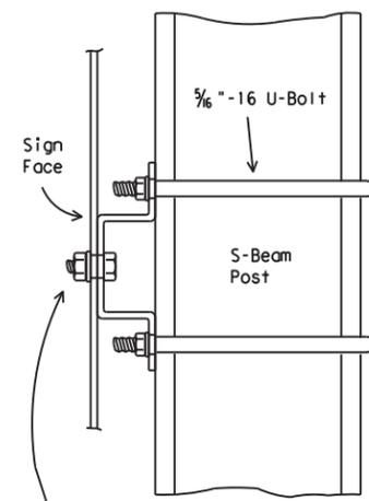
Galvanized steel or aluminum self-locking hex. head nut. 3/8" - 16 x 3/4" hex. head bolt for sheet metal. 3/8" - 16 x 1 1/4" hex. head bolt for plywood. 3/8" galvanized medium washer.
