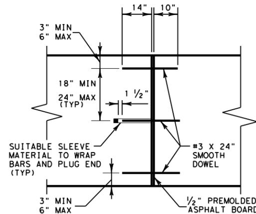
**2 SIDEWALK TRANSVERSE (EXPANSION) JOINT (N.T.S.)**
