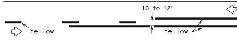
REFLECTORIZED PAVEMENT MARKINGS - PATTERN A
