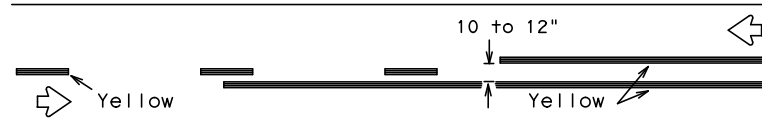
REFLECTORIZED PAVEMENT MARKINGS - PATTERN A
