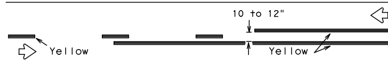
REFLECTORIZED PAVEMENT MARKINGS - PATTERN A
