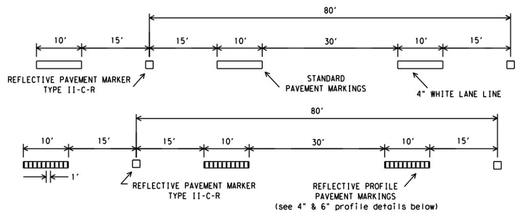
PAVEMENT MARKERS (REFL) TYPE II-C-R SHALL BE SPACED ON 80' CENTERS WITH THE CLEAR FACE TOWARD NORMAL TRAFFIC AND THE RED FACE TOWARD WRONG WAY TRAFFIC.
