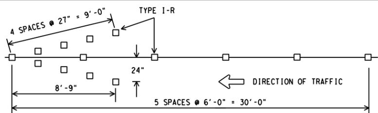
ALL RAISED MARKERS IN THE WRONG WAY ARROW SHALL BE TYPE I-R REFLECTORIZED PAVEMENT MARKERS WITH THE REFLECTORIZED SURFACE FACING THE WRONG WAY TRAFFIC. TYPE II-C-R SHALL NOT BE USED. REFLECTORIZED WRONG WAY ARROWS, NOT TO EXCEED TWO, MAY BE PLACED ON EXIT RAMP. LOCATION OF THE ARROWS SHALL BE AS SHOWN IN THE PLANS OR AS DIRECTED BY THE ENGINEER.
