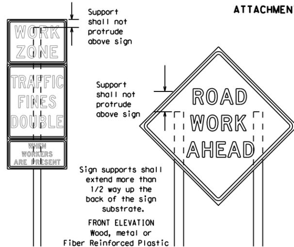
Splicing embedded perforated square metal tubing in order to extend post height will only be allowed when the splice is made using four bolts, two above and two below the splice point. Splice must be located entirely behind the sign substrate, not near the base of the support. Splice insert lengths should be at least 5 times nominal post size, centered on the splice and of at least the same gauge material.
