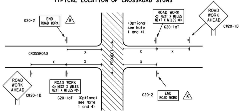
⚠ May be mounted on back of "ROAD WORK AHEAD" (CW20-1D) sign with approval of Engineer. (See note 2 below)
