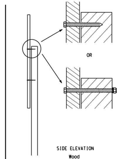
**Nails shall NOT be allowed. Each sign shall be attached directly to the sign support. Multiple signs shall not be joined or spliced by any means. Wood supports shall not be extended or repaired by splicing or other means.**
