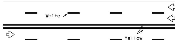
REFLECTORIZED PAVEMENT MARKINGS
