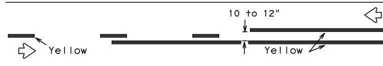
REFLECTORIZED PAVEMENT MARKINGS - PATTERN A
