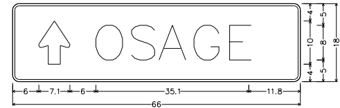
Identifier : D1-1 8in UP; 1.5" Radius, 0.5" Border, White on Green; Standard Arrow Custom 10.0" X 7.1" 90 {}; [OSAGE] ClearviewHwy-3-W;
