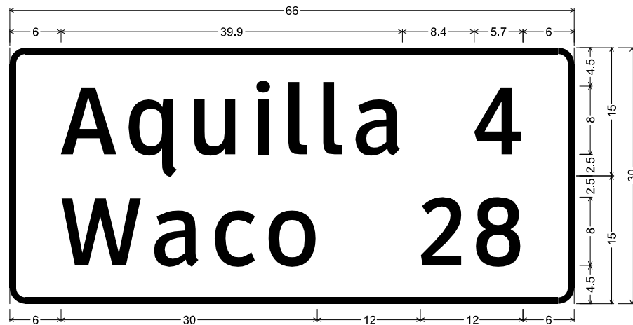
(SIGN 7-1) D2-2 8in; 1.9" Radius, 0.8" Border, White on, Green; "Aquilla", ClearviewHwy-3-W; "4", ClearviewHwy-3-W; 1.9" Radius, 0.8" Border, White on, Green; "Waco", ClearviewHwy-3-W; "28", ClearviewHwy-3-W; (SHEET 7 OF 14)
