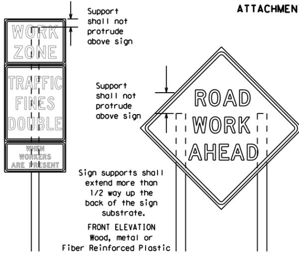
Attachment to wooden supports will be by bolts and nuts or screws. Use TxDOT's or manufacturer's recommended procedures for attaching sign substrates to other types of sign supports
