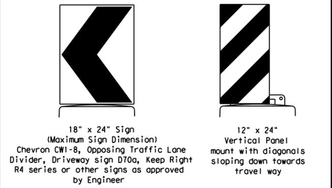
Plywood, Aluminum or Metal sign substrates shall NOT be used on plastic drums
