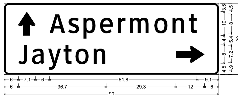
D1-2 8in UP-RT; 1.9" Radius, 0.8" Border, White on, Green; Standard Arrow Custom 10.0" X 7.1" 90°; "Aspermont", ClearviewHwy-3-W; "Jayton", ClearviewHwy-3-W; Standard Arrow Custom 12.0" X 7.1" 0°;
