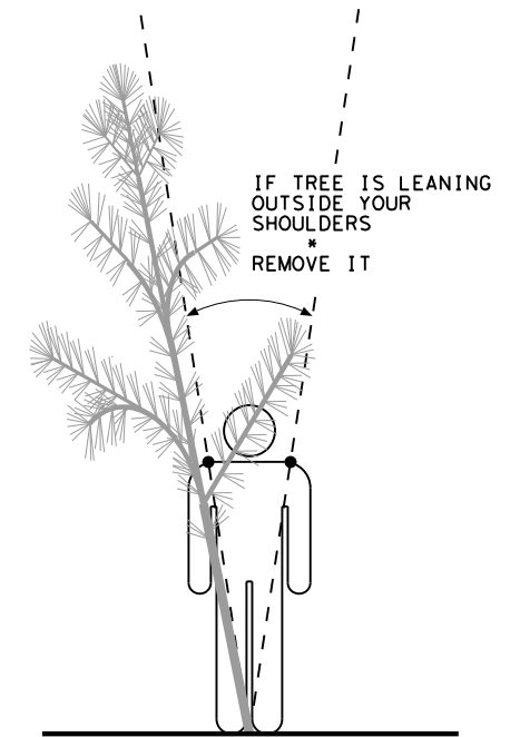
LEANING TREE REMOVAL
