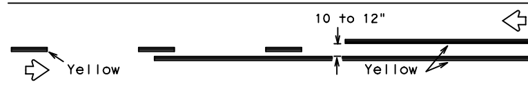
REFLECTORIZED PAVEMENT MARKINGS - PATTERN A
