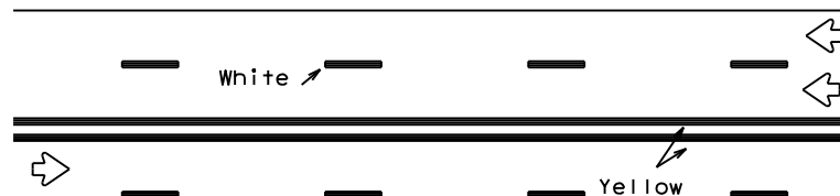
REFLECTORIZED PAVEMENT MARKINGS
