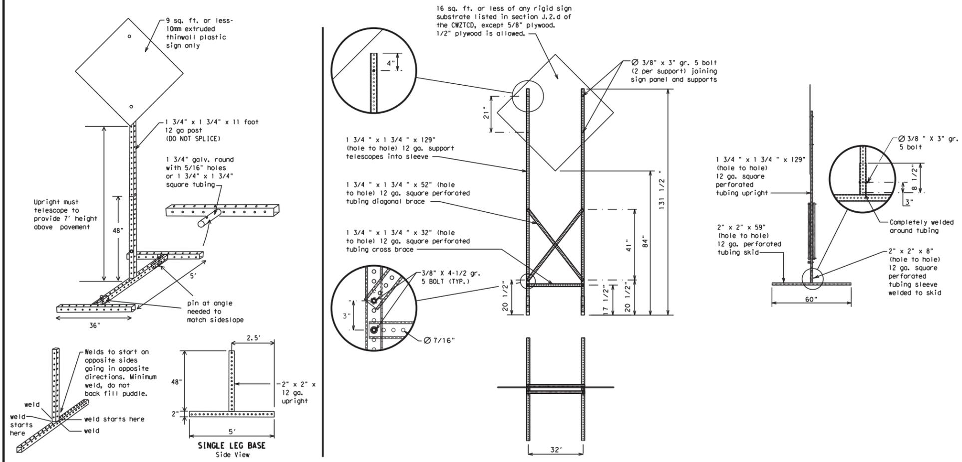
**SKID MOUNTED PERFORATED SQUARE STEEL TUBING SIGN SUPPORTS**
