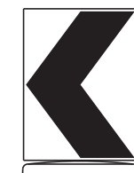
18" x 24" Sign (Maximum Sign Dimension) Chevron CWI-8, Opposing Traffic Lane Divider, Driveway sign D70a, Keep Right R4 series or other signs as approved by Engineer
