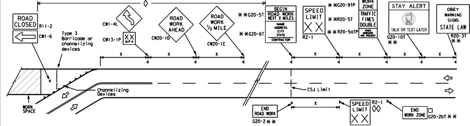
**SAMPLE LAYOUT OF SIGNING FOR WORK BEGINNING AT THE CSJ LIMITS**
