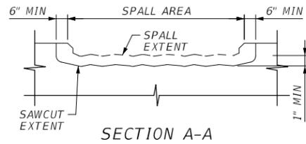
1. SAW-CUT THE AREA AROUND THE SPALL PERIMETER TO SOUND CONCRETE.
