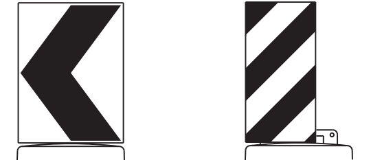
18" x 24" Sign (Maximum Sign Dimension) Chevron CW1-8, Opposing Traffic Lane Divider, Driveway sign D70a, Keep Right R4 series or other signs as approved by Engineer 12" x 24" Vertical Panel mount with diagonals sloping down towards travel way
