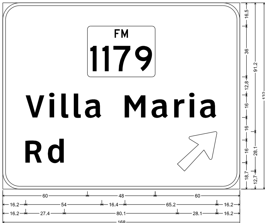
12.0" Radius, 2.0" Border, White on, Green; State Highway 1179 M1-6F4; "Villa Maria", ClearviewHwy-5-W-R; "Rd", ClearviewHwy-5-W-R; Arrow A-3 - 35.6" 45";
