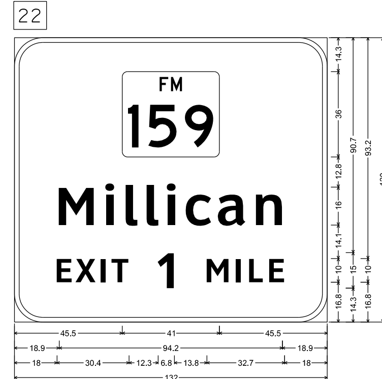
E1-2_VARx120; 12.0" Radius, 2.0" Border, White on, Green; State Highway 159 M1-6F3; "Millican", ClearviewHwy-5-W-R; "EXIT 1 MILE", ClearviewHwy-5-W-R;
