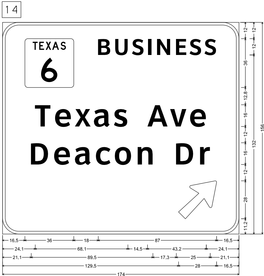
12.0" Radius, 2.0" Border, White on, Green; State Highway 6 M1-6T1; "BUSINESS", ClearviewHwy-5-W-R; "Texas Ave", ClearviewHwy-5-W-R; "Deacon Dr", ClearviewHwy-5-W-R; Arrow A-3 - 35.6" 45';
