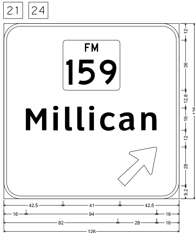
E1-2_VARx120; 12.0" Radius, 2.0" Border, White on, Green; State Highway 159 M1-6F3; "Millican", ClearviewHwy-5-W-R 99% spacing; Arrow A-3 - 35.6" 45';
