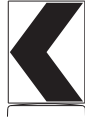
18' x 24' Sign (Maximum Sign Dimension) Chevron (M-8, Opposing Traffic Lane Divider, Driveway Sign D100, Keep Right R4 series or other signs as approved by Engineer)
