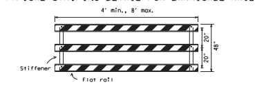
TYPICAL STRIPING DETAIL FOR BARRICADE RAIL TYPICAL PANEL DETAIL FOR SKID OR POST TYPE BARRICADES
