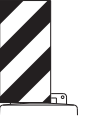
12' x 24' Vertical Panel mount with diagonals sloping down toward travel way Plywood, Aluminum or Metal sign substrates shall NOT be used on plastic drums
