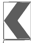
18" x 24" Sign (Maximum Sign Dimension) Chevron CW-8, Opposing Traffic Lane Divider, Driveway sign D70a, Keep Right R4 series or other signs as approved by Engineer
