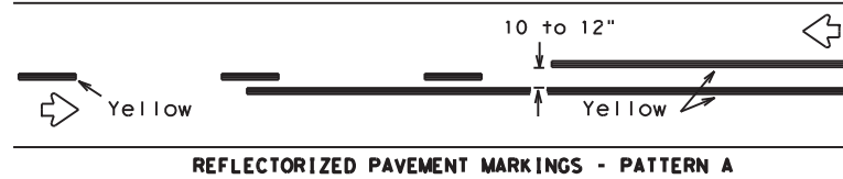
REFLECTORIZED PAVEMENT MARKINGS - PATTERN A
