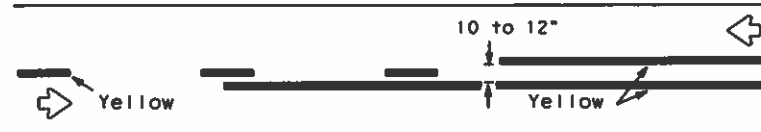
REFLECTORIZED PAVEMENT MARKINGS - PATTERN A
