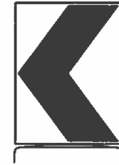
18" x 24" Sign (Maximum Sign Dimension) Chevron CW1-8, Opposing Traffic Lane Divider, Driveway sign D700, Keep Right R4 series or other signs as approved by Engineer
