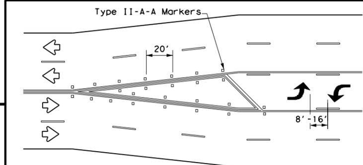
A two-way left-turn (TWLTL) lane-use arrow pavement marking should be used at or just downstream from the beginning of a two-way left-turn lane within a corridor. Repeating the marking after each intersection or dedicated turn bay is not required unless stated elsewhere in the plans.
