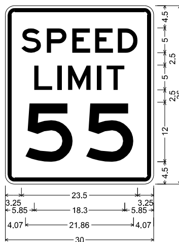
R2-1_30x36; 1.88" Radius, 0.75" Border, 0.50" Indent, Black on, White; "SPEED", E specified length; "LIMIT", E specified length; "55", E specified length;
