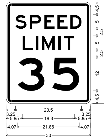
R2-1_30x36; 1.88" Radius, 0.75" Border, 0.50" Indent, Black on, White; "SPEED", E specified length; "LIMIT", E specified length; "35", E specified length;
