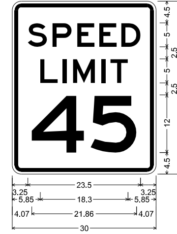
R2-1_30x36; 1.88" Radius, 0.75" Border, 0.50" Indent, Black on, White; "SPEED", E specified length; "LIMIT", E specified length; "45", E specified length;
