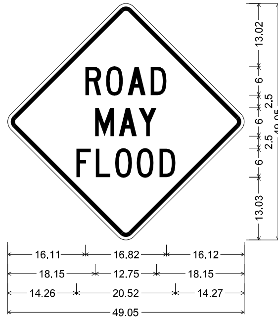
W8-18_36x36; 36.00" across sides 2.25" Radius, 0.88" Border, 0.63" Indent, Black on, Yellow; "ROAD", C; "MAY", C; "FLOOD", C;
