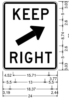
R4-7b_24x30; 1.50" Radius, 0.63" Border, 0.38" Indent, Black on, White; "KEEP", D; Standard Arrow Custom 14.25" X 7.00" 30"; "RIGHT", D;
