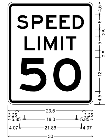
R2-1_30x36; 1.88" Radius, 0.75" Border, 0.50" Indent, Black on, White; "SPEED", E specified length; "LIMIT", E specified length; "50", E specified length;
