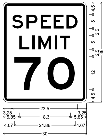
R2-1_30x36; 1.88" Radius, 0.75" Border, 0.50" Indent, Black on, White; "SPEED", E specified length; "LIMIT", E specified length; "70", E specified length;
