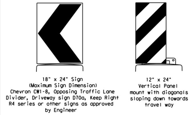
Plywood, Aluminum or Metal sign substrates shall NOT be used on plastic drums
