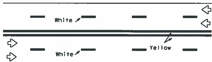
REFLECTORIZED PAVEMENT MARKINGS
