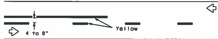
REFLECTORIZED PAVEMENT MARKINGS - PATTERN B
