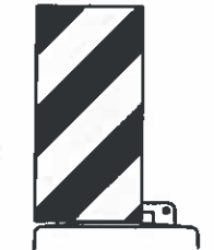
12" x 24" Vertical Panel mount with diagonals sloping down towards travel way
